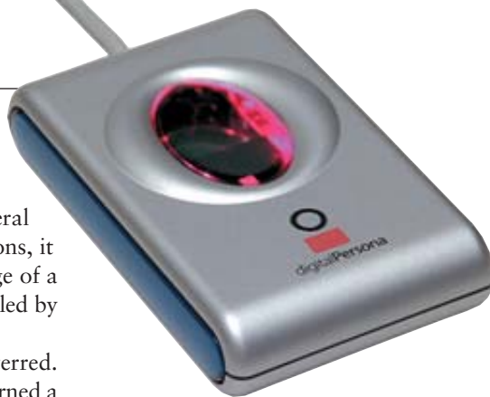
REFLECTED LIGHT reads fingerprint patterns in DigitalPersona's U.are.U 4000 optical sensor.
