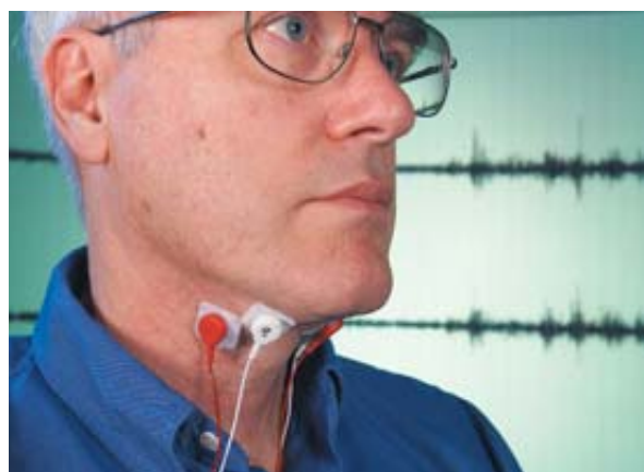
UNSPOKEN TERMS: A computer program and sensors placed near the vocal cords and jaw can pick up silently mouthed words.
