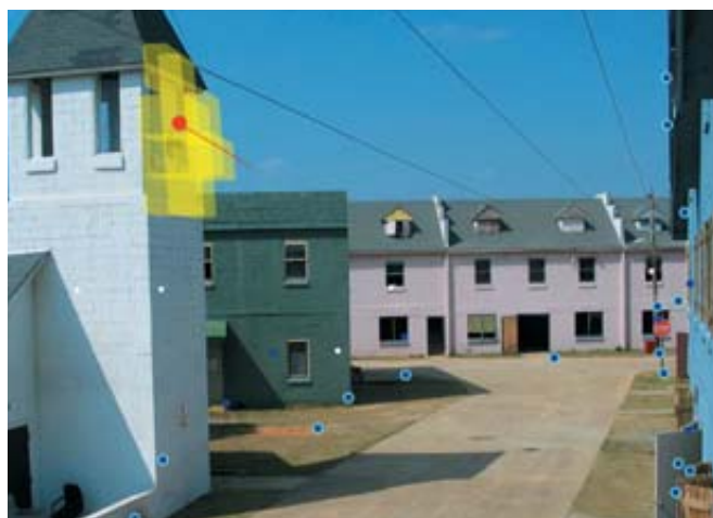
GUNSHOT LOCATION and trajectory (red dot and line) were triangulated within seconds by a network of microphone-equipped motes (blue dots). In tests at Fort Benning, Ga., the system pinpointed rifle shots even when some motes (white dots) had no clear line of sight to the muzzle blast.
